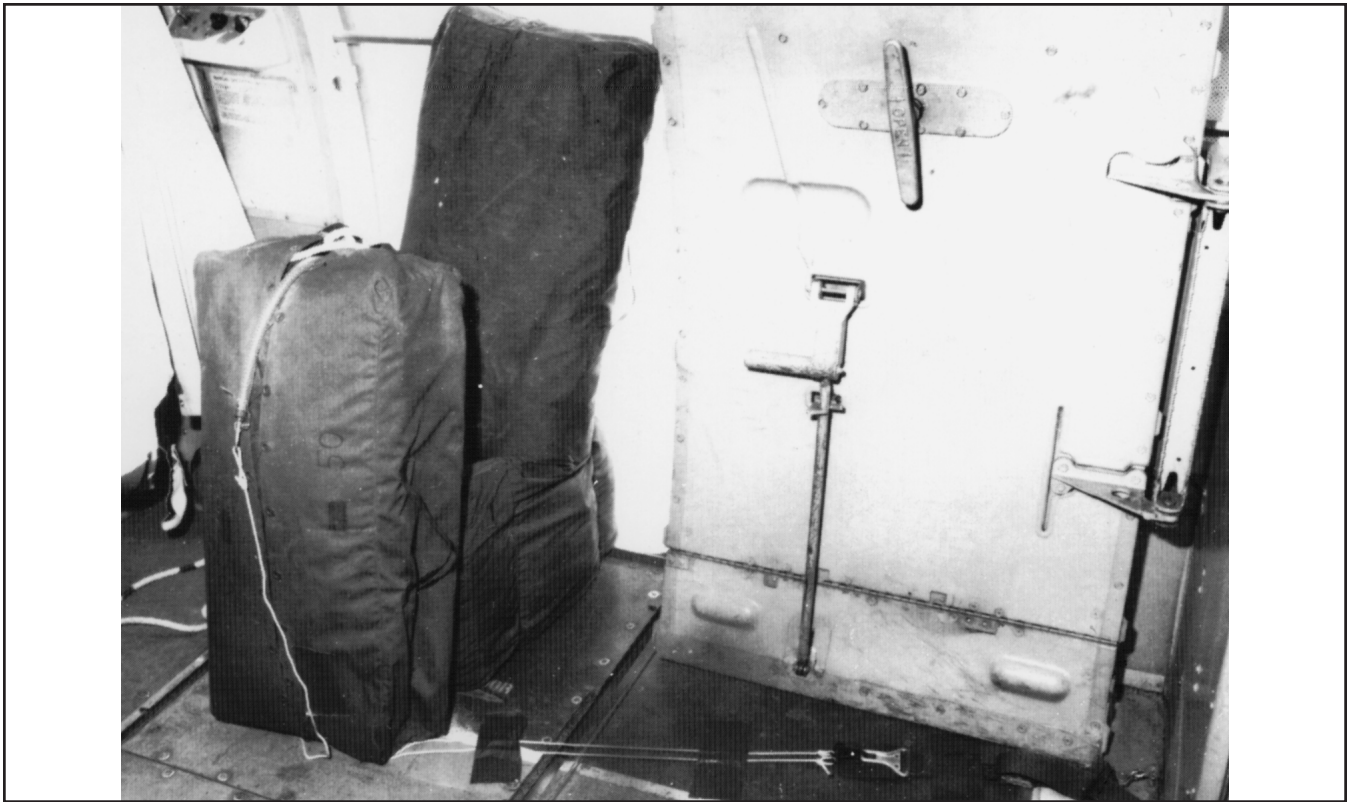
Figure 11-9. SAR Equipment Package Positioning
