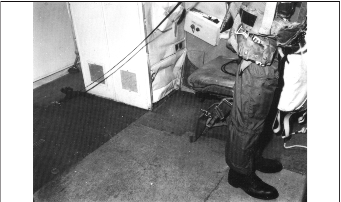
Figure 11-8. Crewmember Safety-Line Attachment
