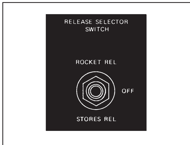
Figure 19-9. Release Selector Switch Panel
