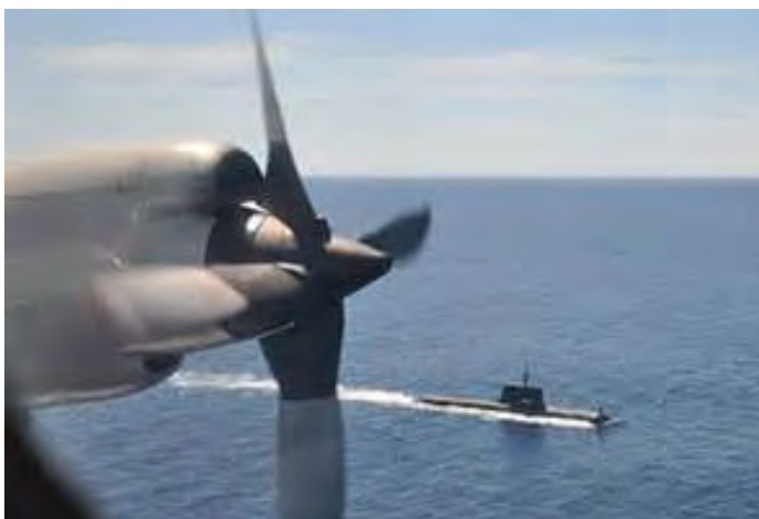
A P-3 onstation with number one engine shut down for loiter.
