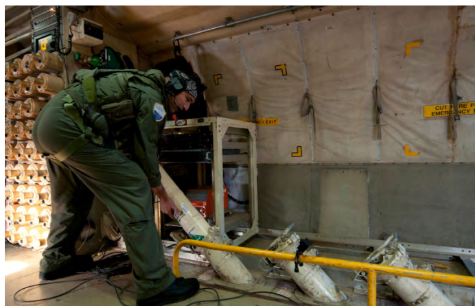
Ordnanceman loading sonobuoys into the "P" (pressure) chutes.
