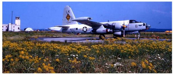
The P2V was a complicated bird. It had two propeller engines and two jet engines with lots of sophisticated sensors for its primary mission, tracking (and attacking if necessary) enemy submarines. (The Trident on the tail was the VP-26 symbol.)
