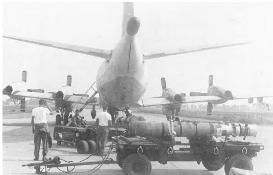
The AO Shop loads MK46 Torpedoes on to a squadron airplane as part of their training evolution.
