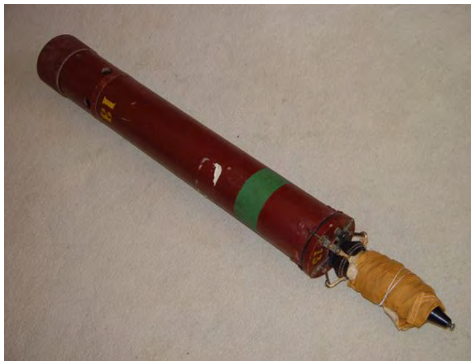
AN/CRT-1 Sonobuoy with hydrophone.
