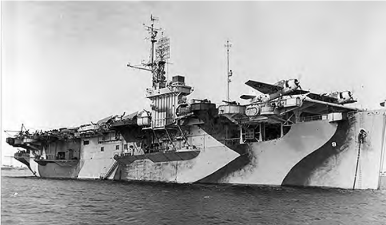
Escort Carrier USS Bogue (CVE-9) in "dazzle" paint with two TBF Avengers up forward.
