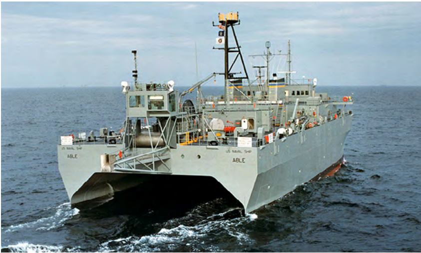
USNS Able (T-AGOS-20). Victorious Class SURTASS ship showing good view of the aft SURTASS deployment equipment.
