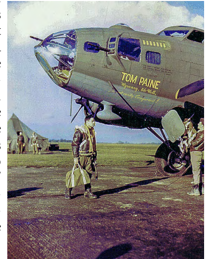
Note the RDF Antenna on the B-17F located in teardrop housing under the nose.
