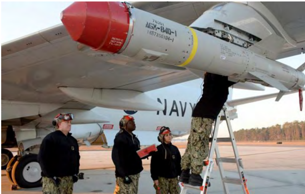
(L to R) AOC Dustin McCuthen, AO1 Derek Torrence and AO2 Alexa Mendez from Patrol Squadron (VP) 45 observe as AO3 Katherine Callahan secures an AGM-84D Harpoon missile to a VP-45 P-8A Poseidon aircraft at Naval Air Station Jacksonville.
