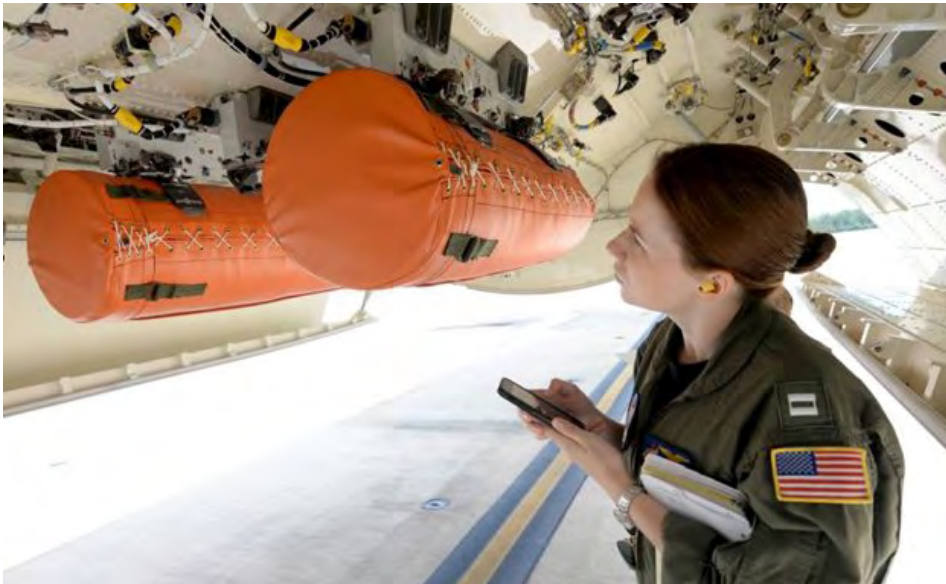
Lt. Laura Ibarra of Patrol Squadron 45, inspects the search and rescue (SAR) kits in the weapon's bay of a P-8A Poseidon before take-off on a mission to Texas in the wake of Hurricane Harvey Aug. 29. This is the first time a SAR kit has been used in a live mission. The kits are large inflatable life rafts with basic survival equipment that are dropped if storm survivors are found in the Gulf of Mexico.
