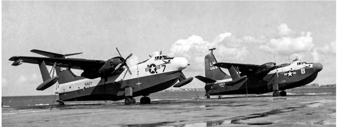
In this 1960 photograph, both P5M versions are parked side by side. LN-7 is a P5M-2 and LN-8 is a P5M-1. Also note the different paint schemes.
