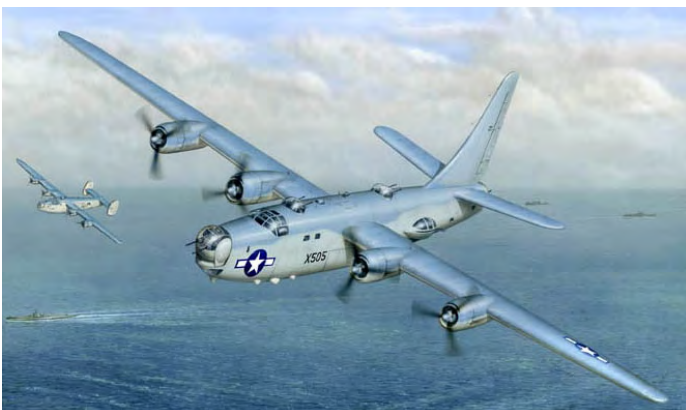
Consolidated's PB4Y-2 Privateer. Similar to the Liberator but a new aircraft for the Navy with single vertical stab, four radials and a flight engineer.
