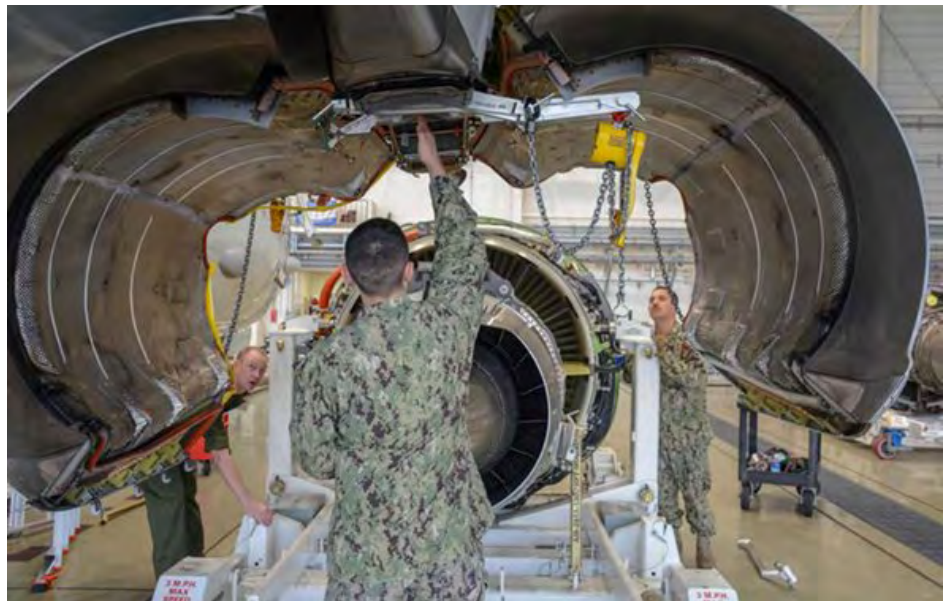
Maintainers of VP-45, replace an engine on a P-8A.
