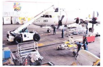
VP-45 Maintenance Team conducts a prop change on the #2 engine
