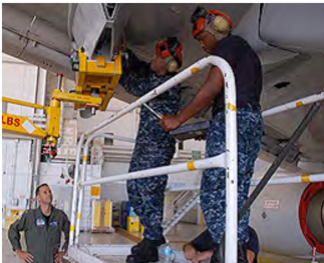
VP-45 Commanding Officer Cmdr. T.J. Grady observes AO2 Chase Dellinger and AO2 Gil Mine as they install a wing rack and pylon onto a P-8A in Hangar 511 at NAS Jacksonville. The Poseidon features four wing pylons and two center line pylons for armament such as the Harpoon anti-ship missile, torpedoes and mines.
