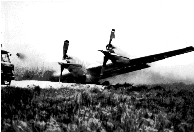
Fuselage and port wing still covered with foam. Though the landing gear had collapsed, both propellers seem to have cleared the terrain.
