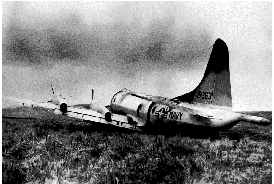
LN-20 at rest with fire out (likely at least a day later). Note that landing gear had collapsed and port wing relatively undamaged.
