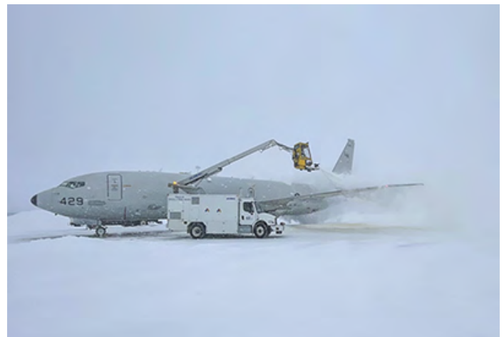
Aircrew conduct De-icing on a P-8 shortly before departure, in the early morning after a snow storm in Misawa
