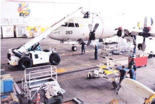
*VP-45 Maintenance Team conducts a prop change on the #2 engine*
